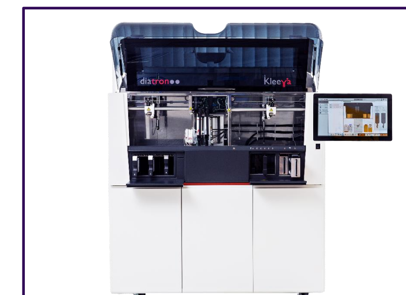
Figure 3. KleeYa® instrument. This assay is performed on the KleeYa® platform (STRATEC SE., Birkenfeld, Germany), a chemiluminescence analyzer that allows for complete automation of an immunoassay. The platform performs the sample processing, reagent dispensing, incubations, wash processes and sample measurement evaluation. The KleeYa® platform is semi-open access, with ALPCO's suite of immunoassay solutions, including our treponemal assay, able to run on a single platform.
