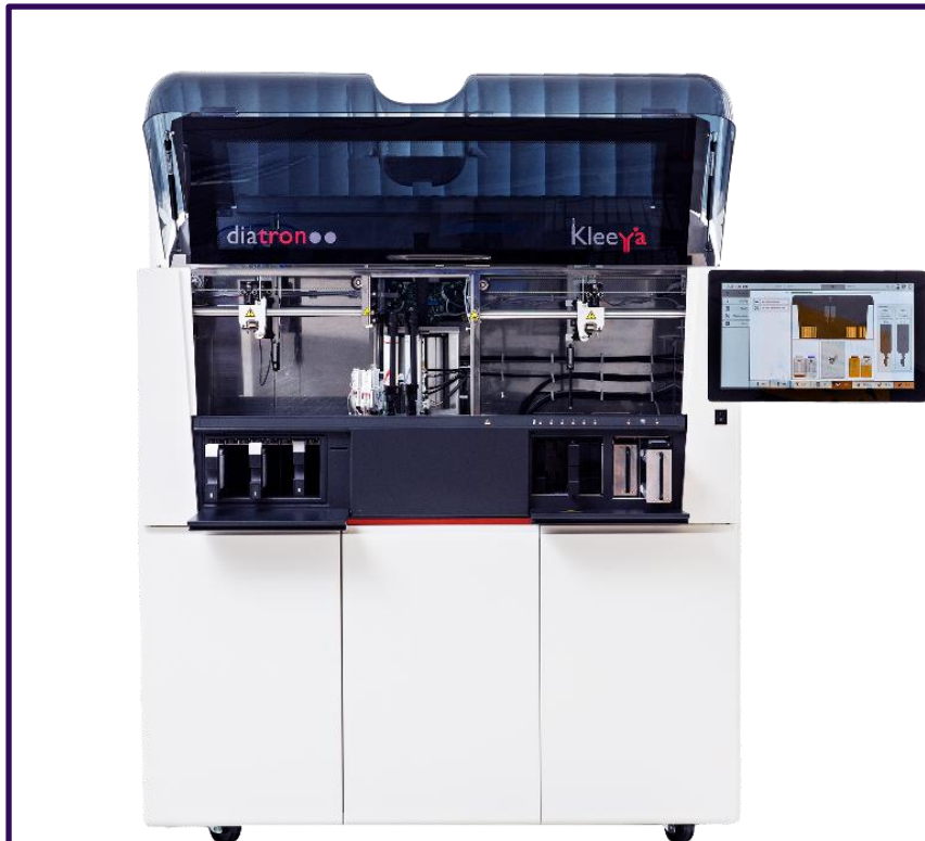
Figure 4. KleeYa ® instrument. These assays are performed on the KleeYa ® platform (STRATEC SE., Birkenfeld, Germany), a chemiluminescence analyzer that allows for complete automation of an immunoassay. The platform performs the sample processing, reagent dispensing, incubations, wash processes and sample measurement evaluation. The KleeYa ® platform is semi-open access, with ALPCO's suite of immunoassays run on a single platform.
